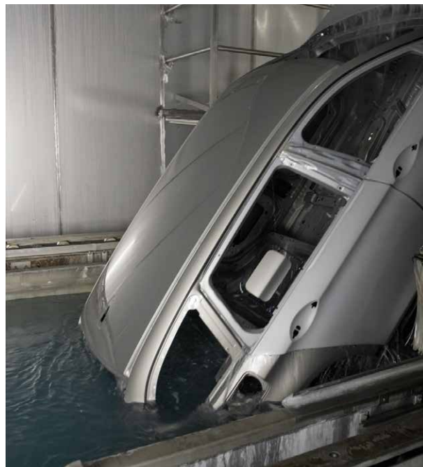
Obr. 4 – Chemetall Dip Tank
